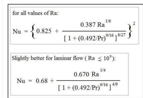
Correlations for Natural Convection Heat Transfer from an Isothermal Vertical Plane
